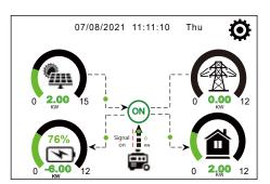
This page tells the PV and diesel generator power the load and battery.
