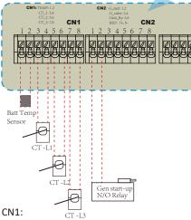
TEMP (1,2): battery temperature sensor for lead acid battery.
