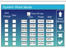
**Time of use:** it is used to program when to use grid or generator to charge the battery, and when to discharge the battery to power the load. Only tick "Time Of Use" then the follow items (Grid, charge, time, power etc.) will take effect.
