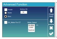
**Ex\_Meter For CT:** when using zero-export to CT mode, the hybrid inverter can select EX\_Meter For CT function and use the different meters.e.g.CHNT and Eastron.
